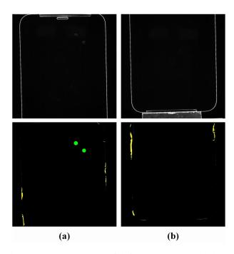
Figure 2: Some examples of defect samples and labels on MSDD-3. The label of "dust" for this dataset is a weakly supervised label, that is, the defective areas are represented by a coarse-grained mask.
