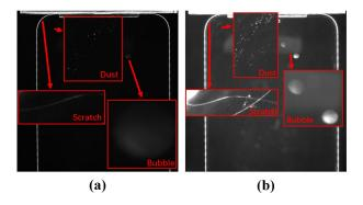
Figure 3: Visualization of highlighted defects. (a) Raw defects. (b) Defects handled by the data Enhancement module.
