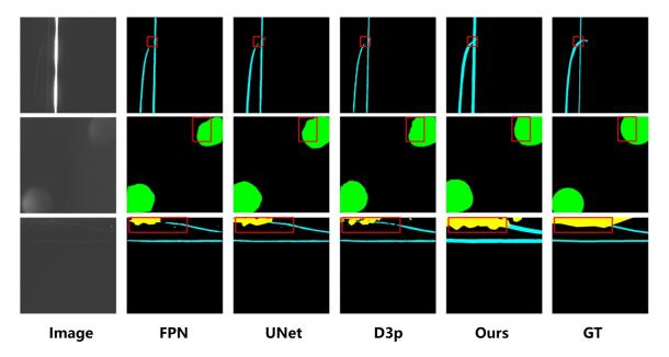
Figure 4: Compared to other methods. Green represents bubbles; Yellow represents the ash layer; Blue is for scratches
